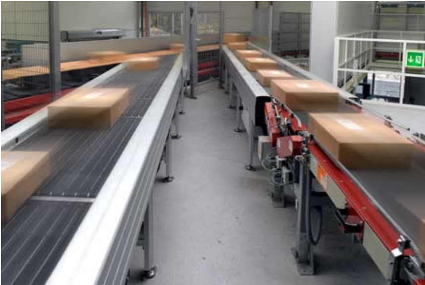
Induction of parcels to the LS-4000E Tilt-Tray shipping sorter
