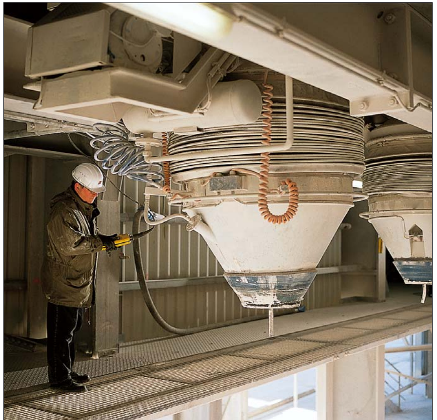
Loading head with integrated filter
