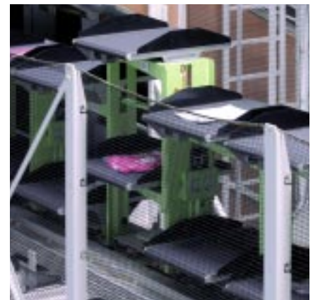
Multi Level Sorter with height-mobile Belt Trays
