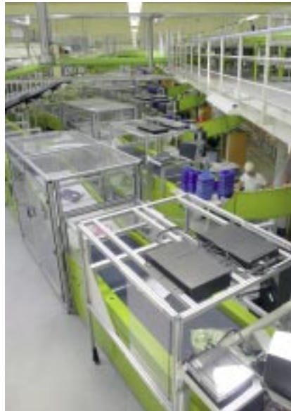
Feed of items on an induction unit, ready for scanning
