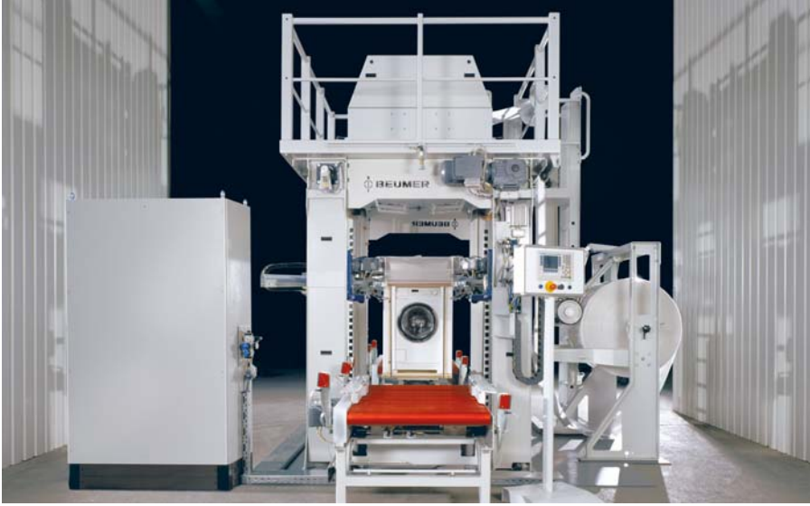
The BEUMER stretch hood® system does not shrink the film.
