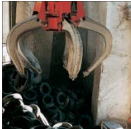
Automatically working gantry crane with polygon gripper for the storage and discharge of scrap tires
